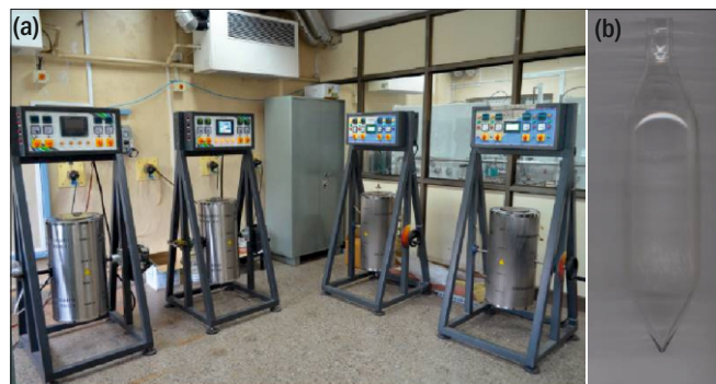
Fig.1:(a) Bridgman furnaces with an operating temperature of 1000°C maximum, located at CTS, TPD used for the growth of halide scintillator single crystals. (b) Quartz crucible used for the growth of CsI single crystal.
